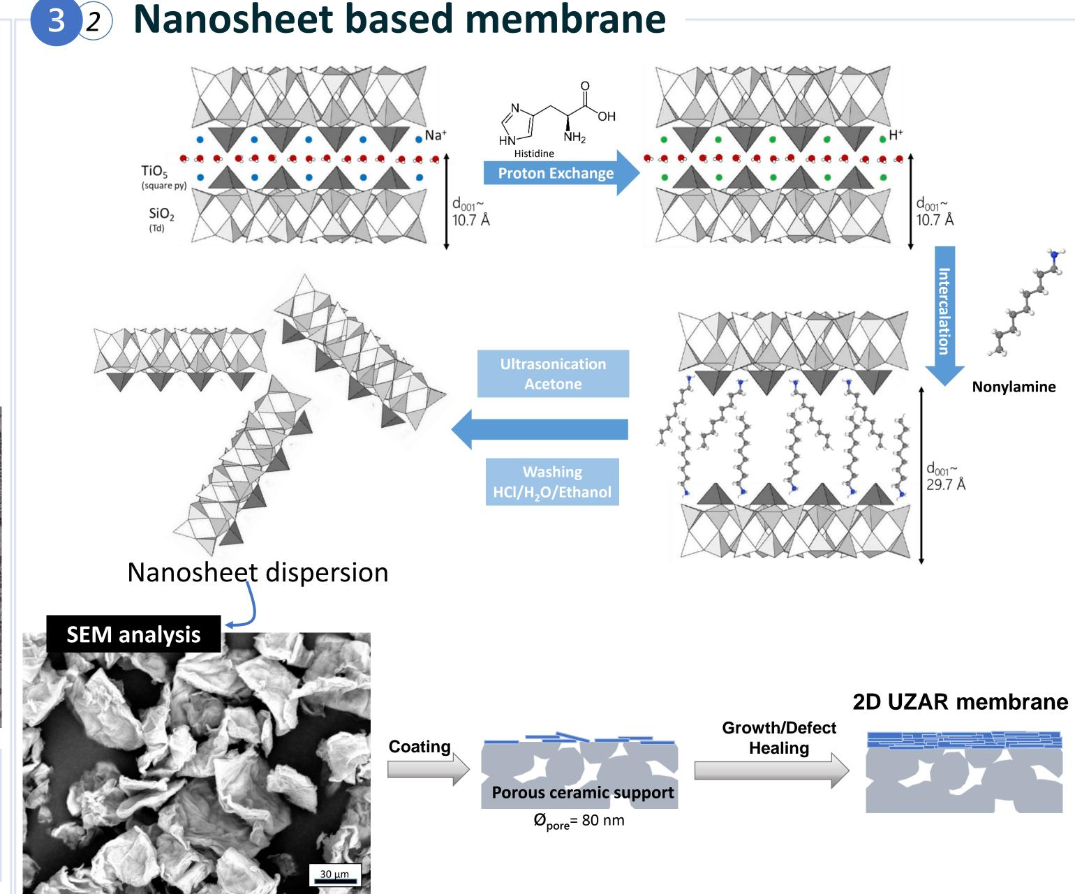
✓ A big challenge in nanosheet science is the creation of a stable nanosheet dispersion. Drying the nanosheets for instance leads to restacking of the sheets. Therefore, the next steps to create a zeolite nanosheet membrane is to create a stable nanosheet dispersion followed by coating the support with the nanosheets.
