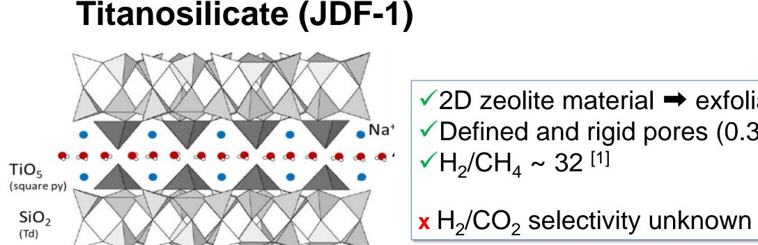
✓ 2D zeolite material → exfoliation possible ✓ Defined and rigid pores (0.3 nm)  $VH_2/CH_4 \sim 32^{[1]}$
