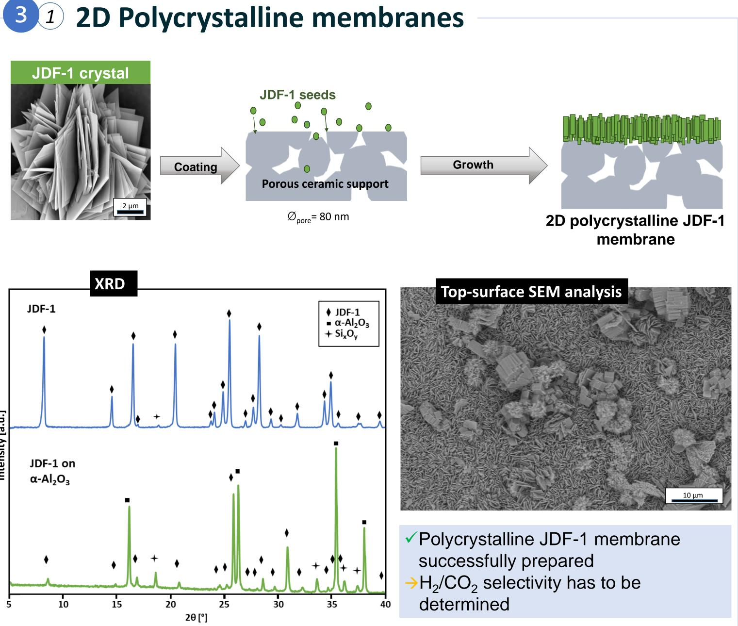
✓ Crystals of JDF-1 were succesfully grown on porous ceramic support. The coverage of the support is highly dependent on the reaction time and can thus be controlled. In the next step, the performance of the as-made membrane will be determined, and the gas separation performance will be improved with the help of post-synthetic methods.
